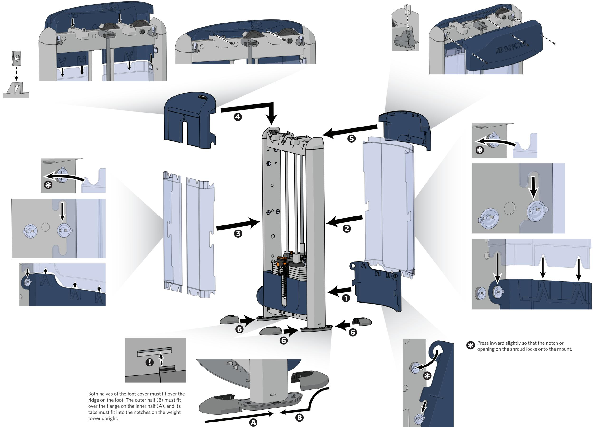
\* Press inward slightly so that the notch or opening on the shroud locks onto the mount.
